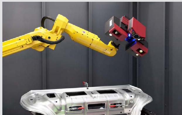
The vision system can detect location, coverage, breaks or gaps, reduced widths, and diagonal breaks. It works on all colors and is fully adjustable to meet each customer's specifications. These systems are highly customized to particular design and manufacturing requirements. Sika's System Engineering Department can provide guidance for system integrators.
