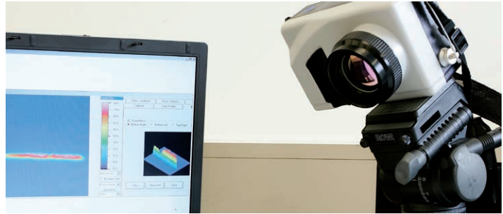
Sika System Engineering supports the optimization of the adhesive application by patented test methods. The above image shows an infrared camera measuring the adhesives heat of reaction.
