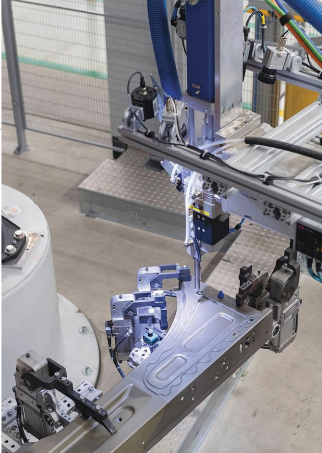
Typical application of epoxy body shop adhesive during assembly process.
